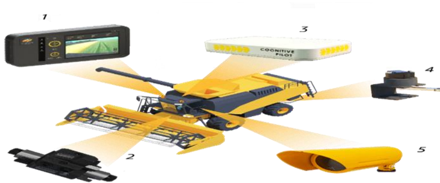
Figure (1) Parts of the system and their installation locations in the harvester
